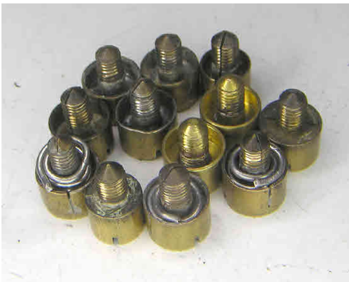
This is interesting. At least eight of the screws have either been hot soldered or have twists of solder added to them. This must be to add weight and slow the clock down. The hot soldered screws will be the most difficult to correct and clean up without leaving marks.
