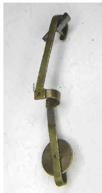
The fibre block that carries the contact flag terminal has been broken and filled with plastic filler. The soldered connection is also very poor.
