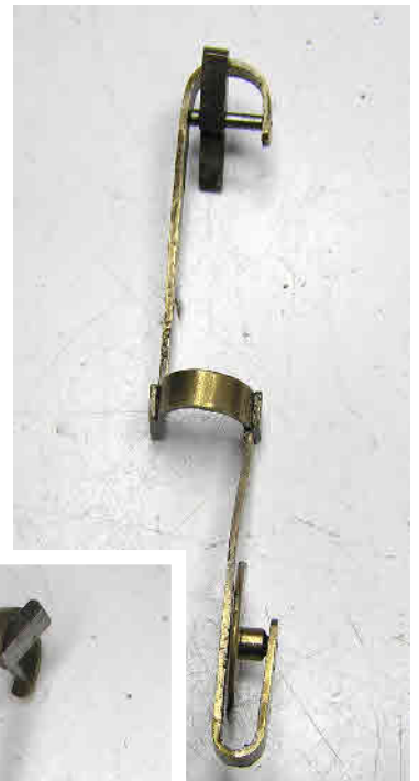
The rear pivot bearing housing also shows signs of rust with the pivot boring a hole in the glass. The impulse arm shown below, is complete if rather a little battered.
