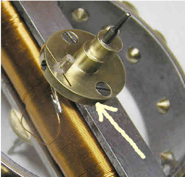
The new front pivot assembly in place on the cleaned and balanced wheel.
