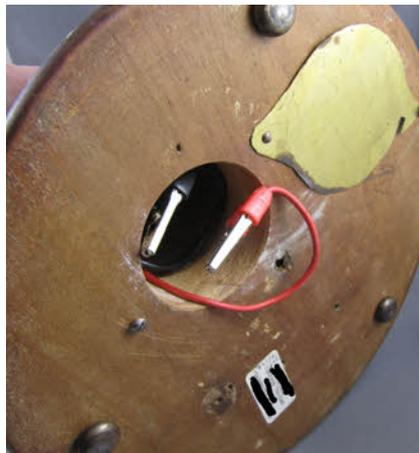
*This photo shows the bottom of the base which has small bun feet and no height adjusting screw. Note also the rough poorly made brass battery cover.*
