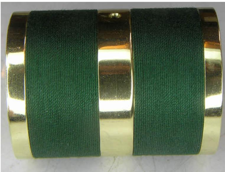
*The coil casing after cleaning and winding with green cord.*
