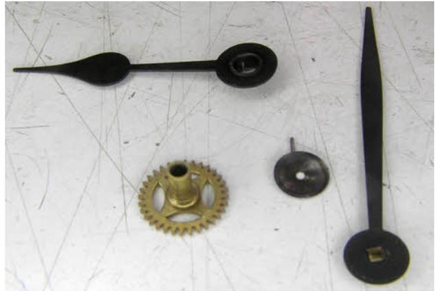
Above can be seen the replacement hands and a replacement hour motion wheel. All will be replaced. Below shows the rear of the movement and the missing Contact spring.
