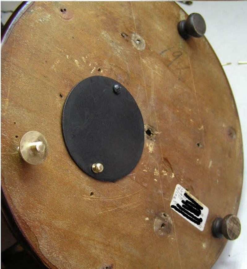
*These photos shows the base after cleaning, filling and polishing. The steel feet have been replaced with wooden bun type feet and levelling screw. The new battery cover has been fashioned from plate steel as per the original. So although the base is a replacement, it is now more in line with an original Bulle base allowing the clock to be levelled on uneven surfaces.*
