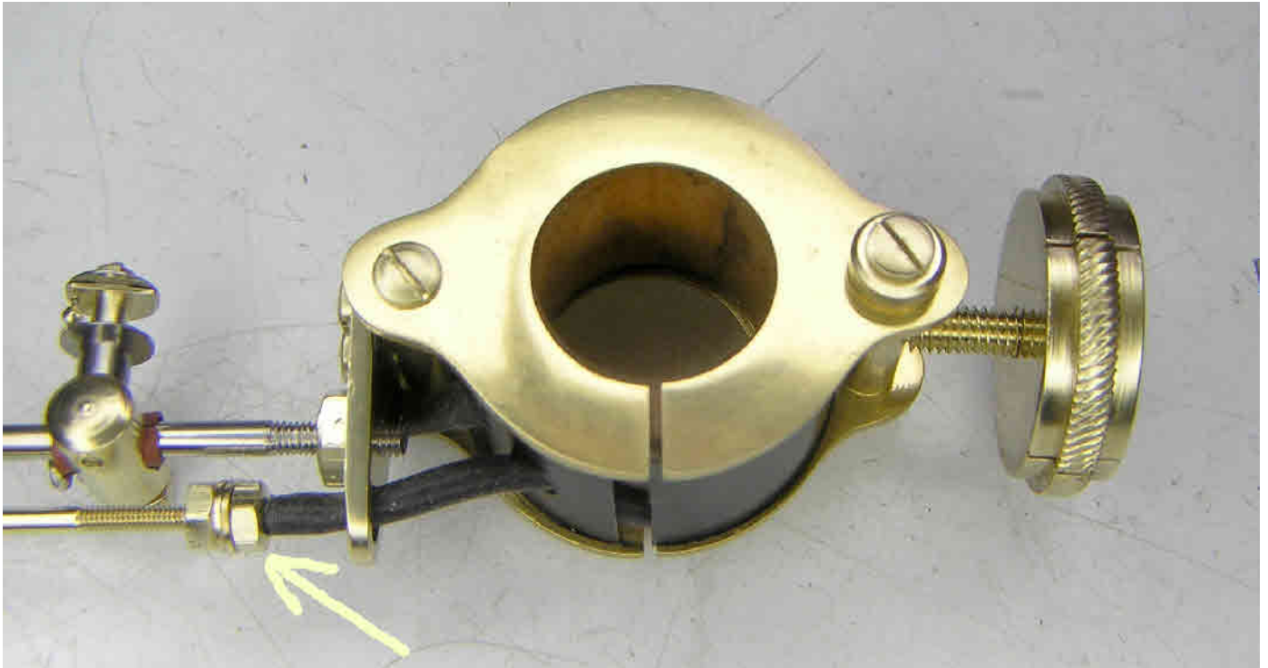
The completed coil assembly with new lead out wire back in place with the pendulum. Note how the wire is insulated from the pendulum rod and casing. It is then attached via the two nuts to the screwed rod carrying the power back up to the contact pin.
