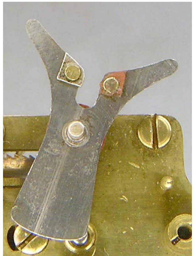
The movement itself is complete and in good condition. The fork fibre insulator is very worn and needs replacing. The silver contact though is pretty good with hardly any wear on the inside, so it will be kept. All the assemblies can now be stripped and cleaned.
