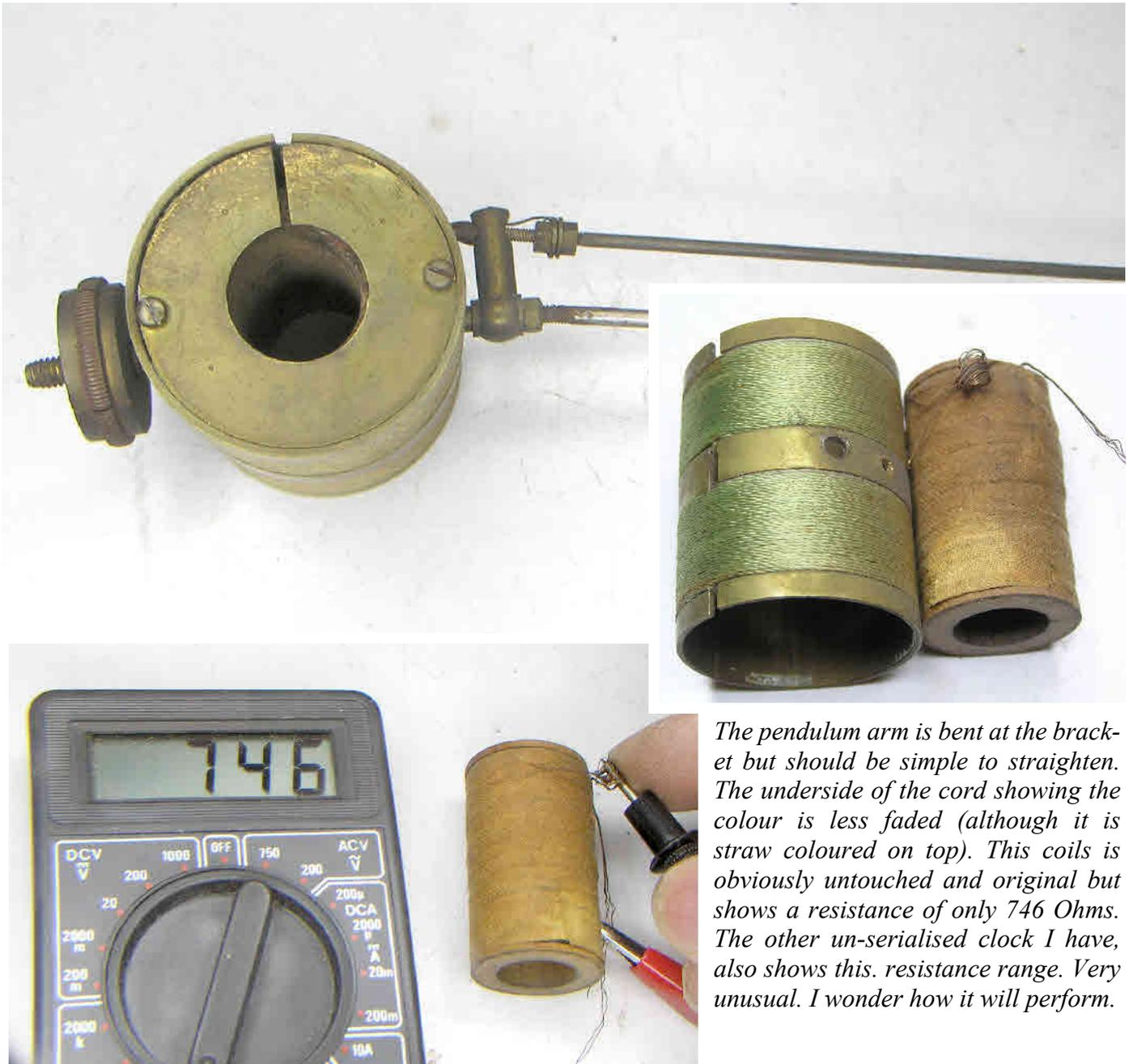
*The pendulum arm is bent at the bracket but should be simple to straighten. The underside of the cord showing the colour is less faded (although it is straw coloured on top). This coils is obviously untouched and original but shows a resistance of only 746 Ohms. The other un-serialised clock I have, also shows this. resistance range. Very unusual. I wonder how it will perform.*
