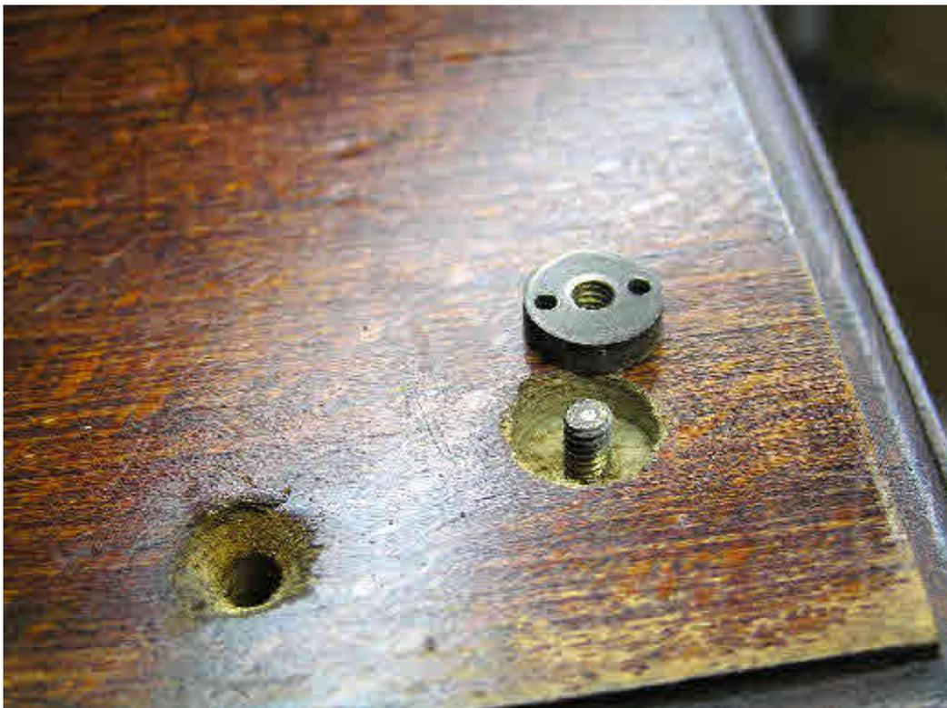
*The front of the case is held together by brass tie rods that are pushed all the way through the case to protrude in counter bored holes. These threaded ends are then captured by threaded washers with two 1.5mm driving holes. The glass is held in place by slotted wood beads with brass angle to cover the plate ends.*
