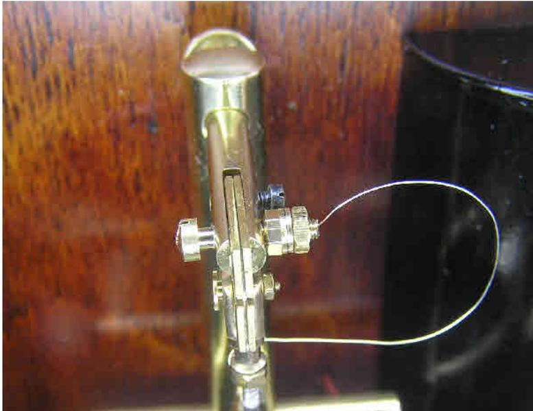
*The suspension assembly with it's new nuts and bolts. These earlier pendulums did not have the small screw and washers with which the contact wire was secured to the top of the pendulum. Instead the wire was captured by the nut that locked the lower suspension bracket to the top of the steel pendulum rod.
