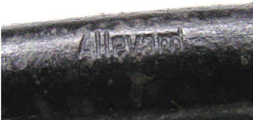
*This original bar magnet is in good condition and gives a reading of 160mm on my home made magnetometer. This is just a little lower than I would normally accept so I re-magnetised it to read 190mm. It is stamped with what could be the manufacturer's name - "Allevam", "Allevard" or even "Allevam". But the most probable explanation is that it is the name of the town where iron and steel were produced at the end of the 19th and beginning of the 20th century - Allevard in South East France*
