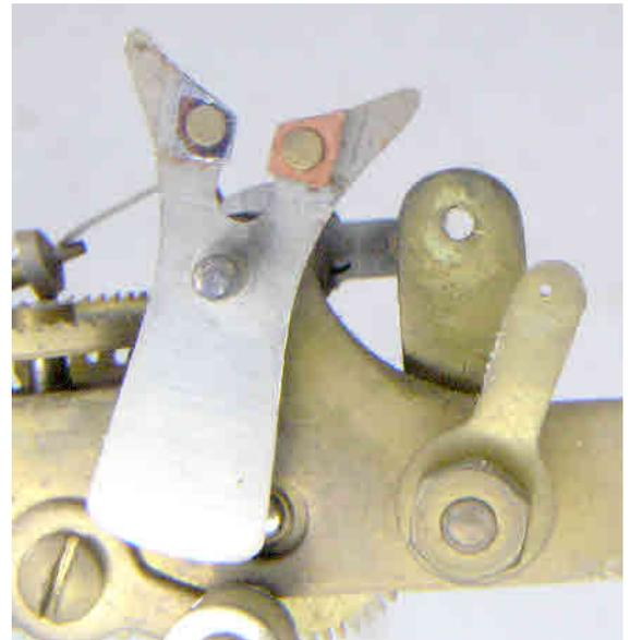
*The suspension itself is missing as well as the all the nuts and screws of the assembly. These will need to be manufactured.*
