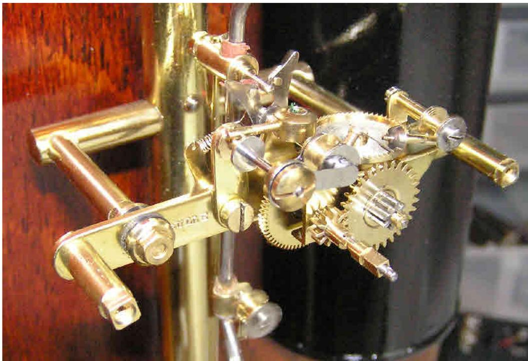
The movement reassembled with the new fork contacts and silver contact
