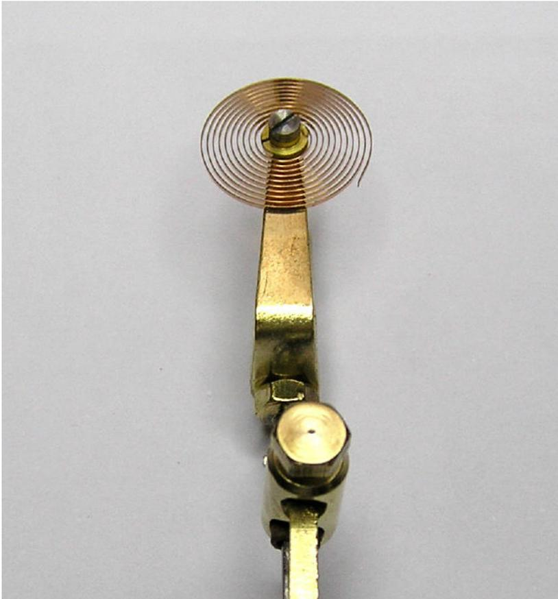
*As I first suspected on seeing this clock very little was damaged or missing. So apart from the Balance contact spring and the Fork contacts the rest of the clock was in good order and just needed a strip and clean. These photos show the new spring and the finished pendulum about to be re-united with the dial plate.*
