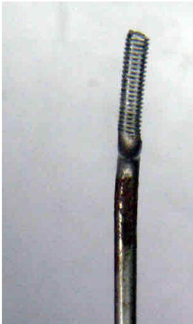
These two photos show the top of the pendulum rod before and after straightening..
