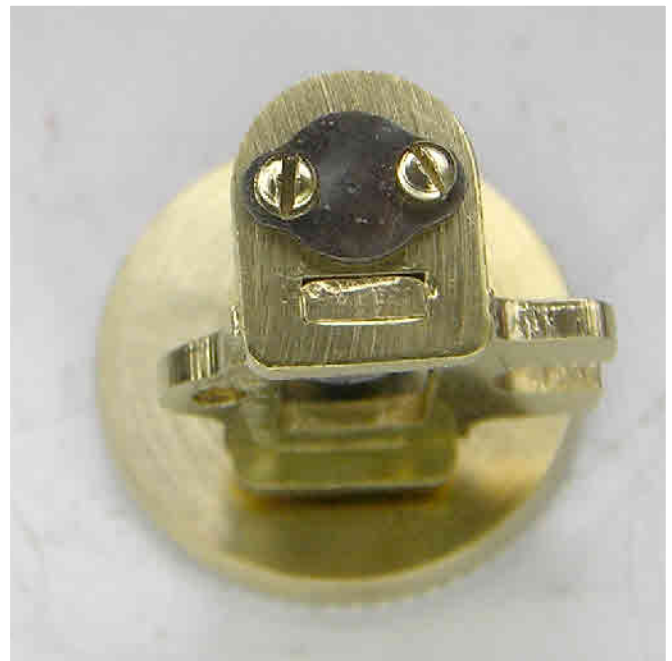
The photo above shows the new end stop plate for the count wheel. Note that this design has two screws. The original plate must have gone walkabout at some time in the past and a plate from different movement used as a replacement.
