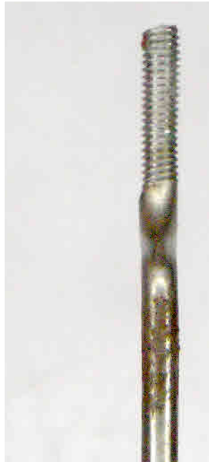
These two photos show the top of the pendulum rod before and after straightening..
